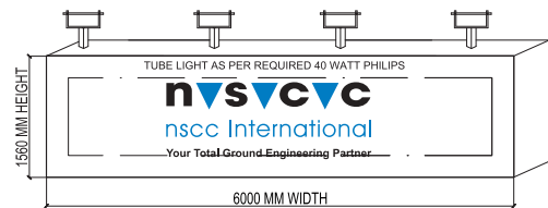
TOWER CRANE LIGHT BOX 3D SCALE 1:100
